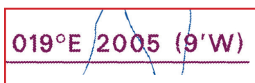
Fig. 2.27 Typical characteristics of the Magnetic Variation as given on the chart's compass rose. In 2005, Magnetic Variation, in this area, was 19° East, decreasing by 9' every year (extracted from Fig. 2.26).
