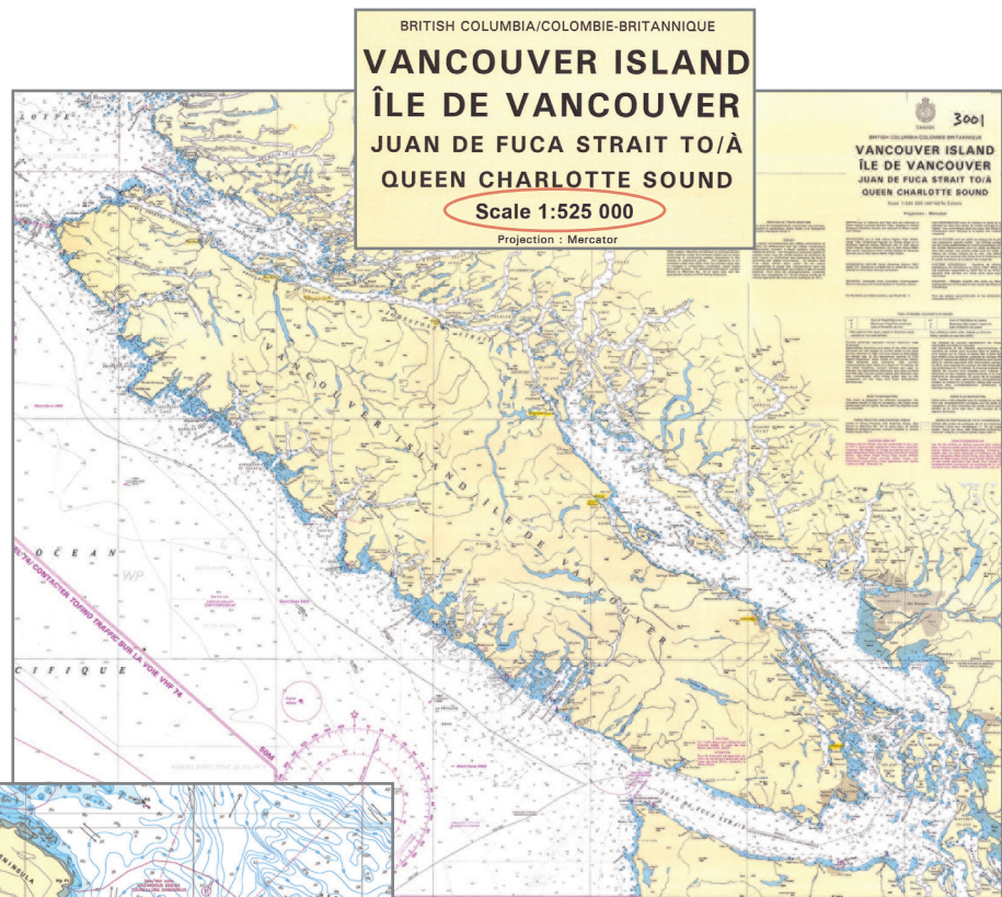
Fig. 2.7 Chart 3001, Small Scale (1/525,000). Used for initial (overall) planning of a cruise.
