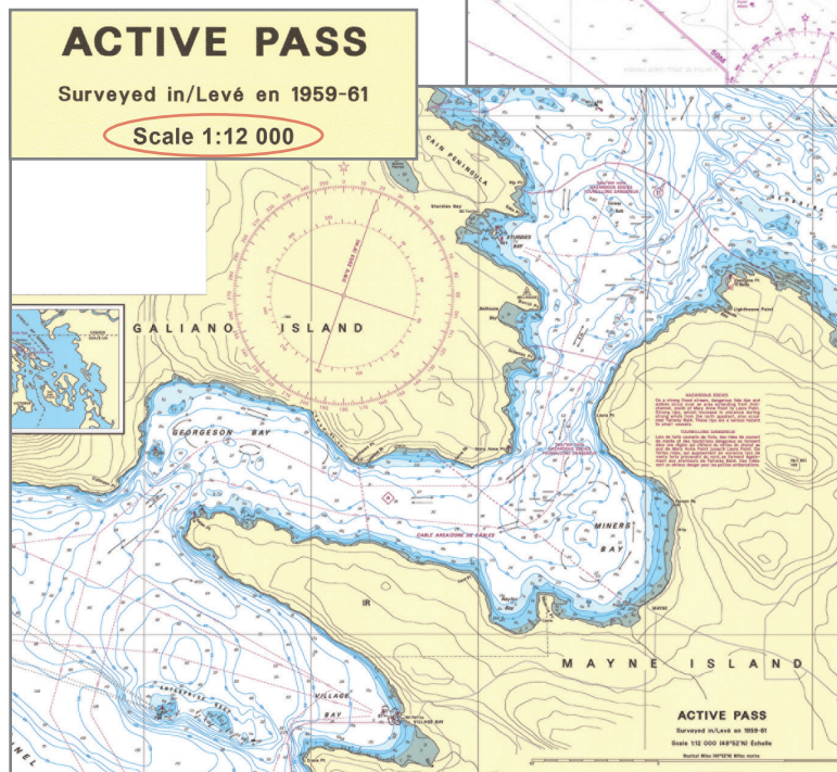
Fig. 2.8 Chart 3473, Large Scale (1/12,000). Used for detailed passage planning.
