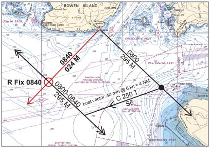
Fig. 11.16 Step 6: Draw LOP 2 at 08:40, and determine the fix at 08:40.
