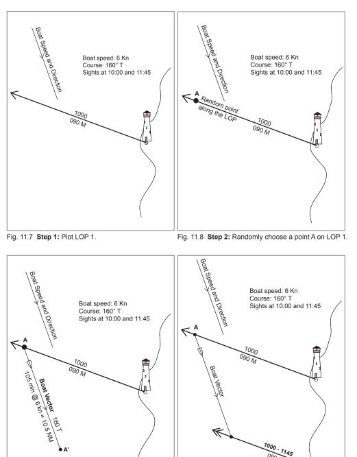
Fig. 11.9 **Step 3:** From A, plot the Boat Vector for the time interval between the first and the second sights.
