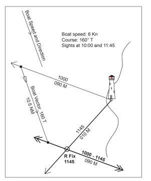
Fig. 11.11 **Step 5:** Plot LOP 2, and determine the boat position at the time of sight 2.
