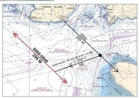
Fig. 11.15 Step 5: Advance the first LOP from 08:00 to 08:40.
