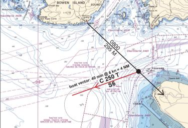
Fig. 11.14 **Step 4:** Draw the Boat Vector for 40 min (from 08:00 to 08:40).
