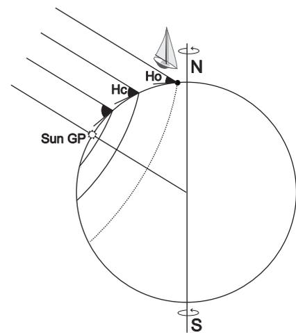
Fig. 1.8 Circles of Position for various **altitudes**  $H$  of a celestial object over the horizon. The further away the observer is from the GP, the lower the object's altitude over the horizon.
