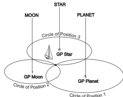
Fig 1.3 A fixed observer can directly use two or three lines (circles) of position from different celestial objects at the same time.
