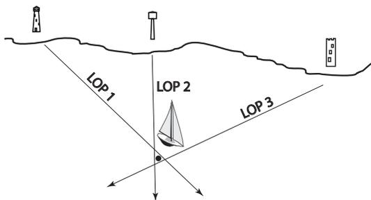
Fig. 1.1 Traditional fix, using three bearings on three landmarks.
