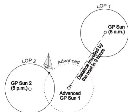
Fig. 1.5 A moving observer needs to **advance** the first line (circle) of position by the distance traveled between the two observations, thus obtaining a Running Fix.
