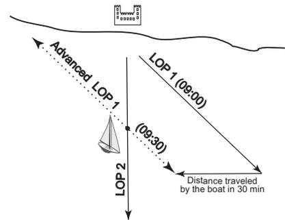
Fig 1.2 Running Fix (Advanced Line of Position), using two bearings on a single landmark.
