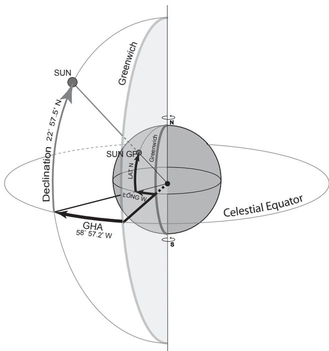
Fig. 1.6 These celestial coordinates are equivalent to the ones on the surface of the earth (Lat. 22° 57.5' N, Long. 58° 57.2' W).
