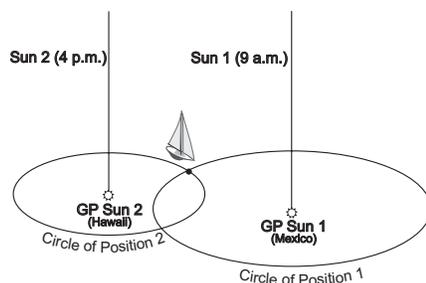
Fig 1.4 A fixed observer can directly use two lines (circles) of position from the same object at different times.
