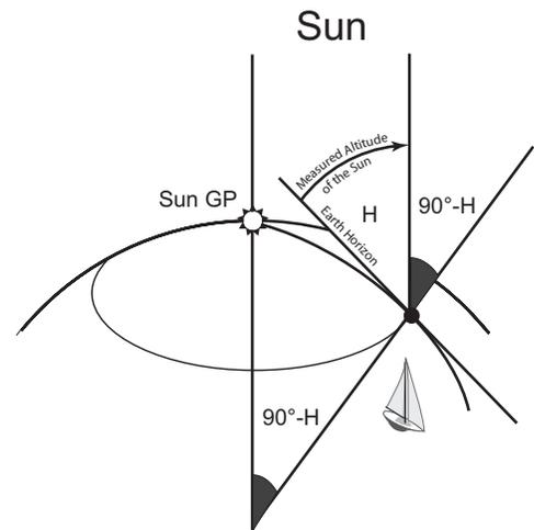
Fig. 1.9 The angle at the Center of the Earth ( $90^\circ - H$ ) is equal to the Zenith Distance, i.e.  $90^\circ$  minus the altitude ( $H$ ) of the sun above the horizon.
