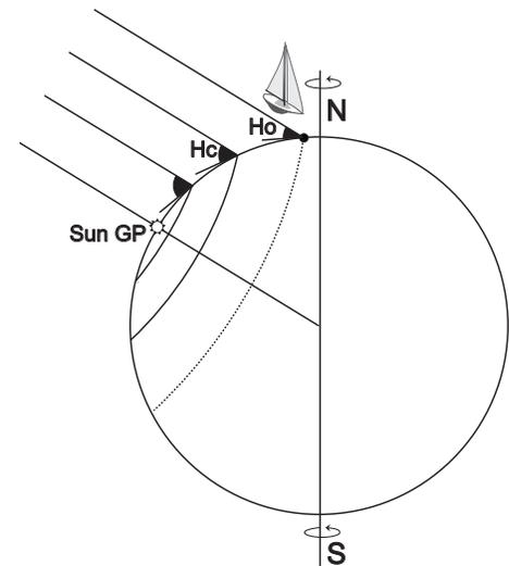
Fig. 1.10 The angle at the Center of the Earth ( $90^\circ - H$ ) allows drawing a Circle of Position, at least in theory.
