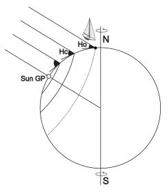
Fig. 1.10 The angle at the Center of the Earth (90 $^{\circ}$  – H) allows drawing a Circle of Position, at least in theory.
