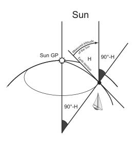
Fig. 1.9 The angle at the Center of the Earth  $(90^{\circ} - H)$  is equal to the Zenith Distance, i.e.  $90^{\circ}$  minus the altitude (H) of the sun above the horizon.
