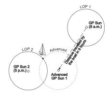
Fig. 1.5 A moving observer needs to **advance** the first line (circle) of position by the distance traveled between the two observations, thus obtaining a Running Fix.
