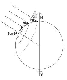
Fig. 1.8 Circles of Position for various **altitudes** H of a celestial object over the horizon. The further away the observer is from the GP, the lower the object's altitude over the horizon.
