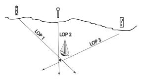
Fig. 1.1 Traditional fix, using three bearings on three landmarks.
