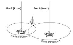
Fig 1.4 A fixed observer can directly use two lines (circles) of position from the same object at different times.
