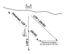
Fig 1.2 Running Fix (Advanced Line of Position), using two bearings on a single landmark.
