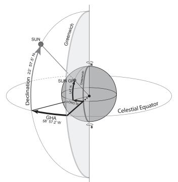
Fig. 1.6 These celestial coordinates are equivalent to the ones on the surface of the earth (Lat. 22° 57.5' N, Long. 58°57.2' W).
