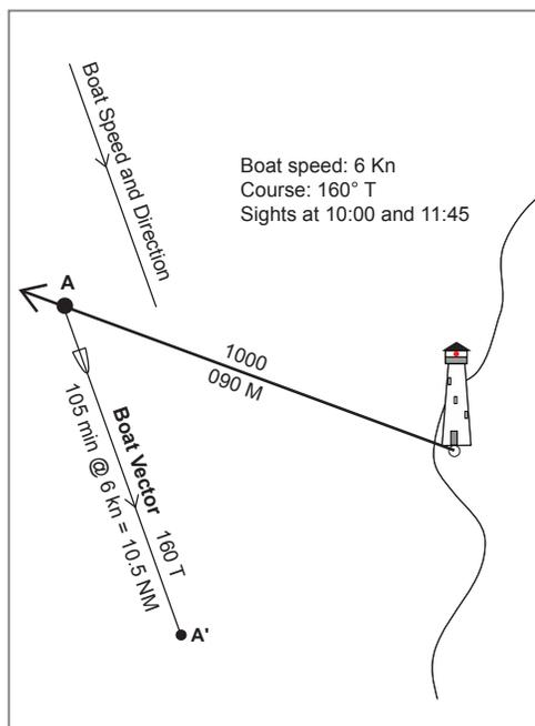
Fig. 11.9 **Step 3:** From A, plot the Boat Vector for the time interval between the first and the second sights.
