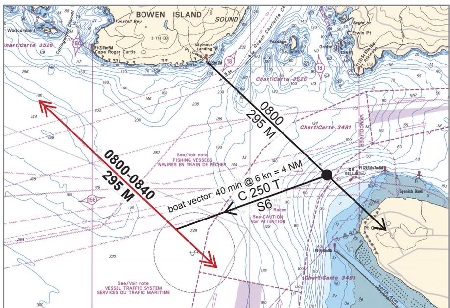
Fig. 11.15 Step 5: Advance the first LOP from 08:00 to 08:40.
