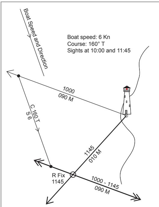
Fig. 11.17 Labeling of Advanced Lines of Position. On this graphic, boat direction (c) = 160° T; boat speed (s) = 6 kn.
