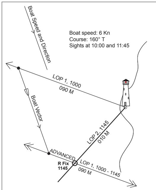
Fig. 11.6 LOP 2 at 11:45, and Running Fix at 11:45.
