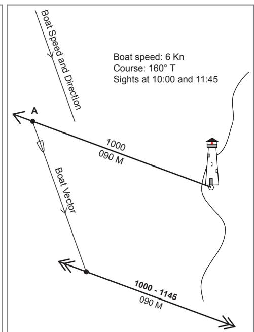
Fig. 11.10 **Step 4:** From the tip of the Boat Vector, draw a parallel to LOP 1.
