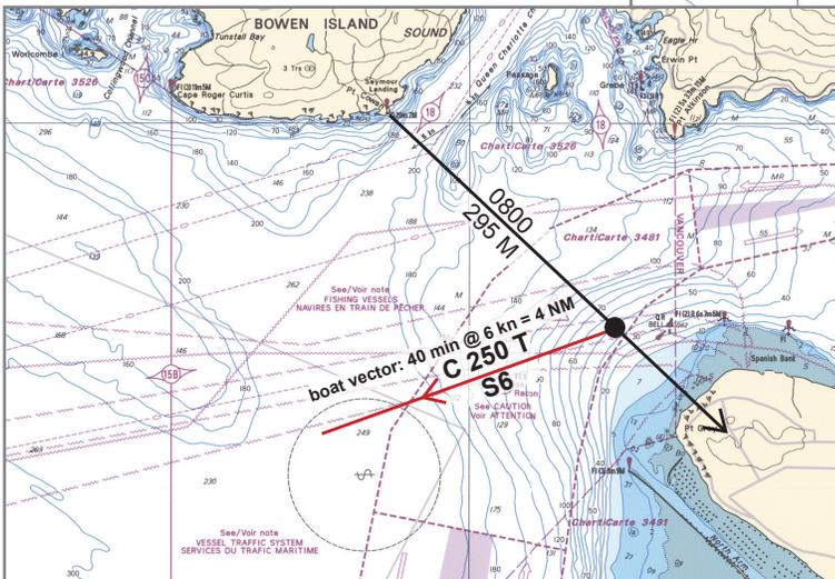
Fig. 11.14 Step 4: Draw the Boat Vector for 40 min (from 08:00 to 08:40).
